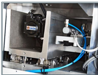
Rear view of the Versamill 4X-100 showing cast aluminum-alloy castings linear guide ways
