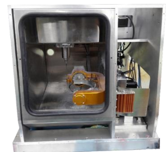
Aluminum frames, while offering strength and rigidity provide less vibration dampening than cast machine frames.
